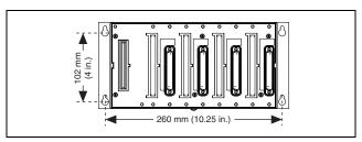
Figure 10. Dimensions of Compact FieldPoint Horizontal Panel-Mount Kit Installed on cFP-BP-4
